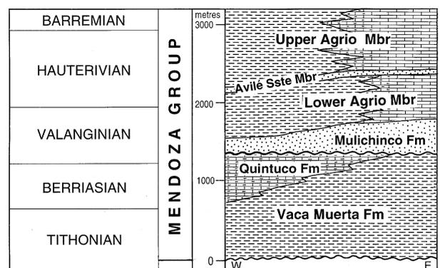
Figure 3. Schematic stratigraphic section of the Mendoza Group.
